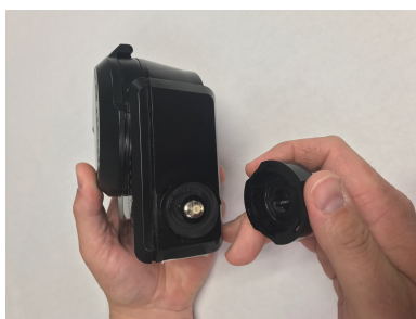
Figure 9 – Remove the Protective Cap and Gasket
