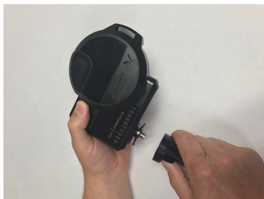
Figure 10 – Align the F Connector
