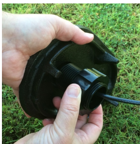
Figure 7 – Secure the Locking Nut
