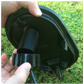
Figure 6 – Locking Nut on Antenna
