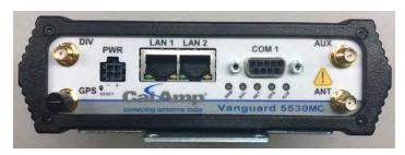
Figure 94 – Modem Front View
