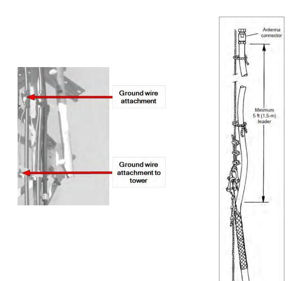
The following images are examples of the coaxial ground kit and coaxial hoisting grips.
