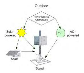
The gateway mounted on a stand can be either solar-powered or AC-powered.
