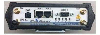
Figure 104 – Cellular Modem Front - Status LEDs
