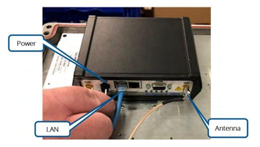
Figure 112 – Disconnect Power, Ethernet, and Antenna Cable
