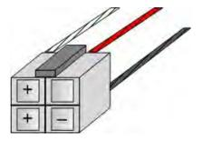
Figure 96 – Cellular Modem Power Plug
