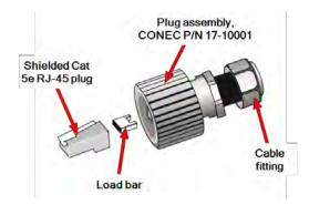
Figure 87 - Feed-Through Assembly
