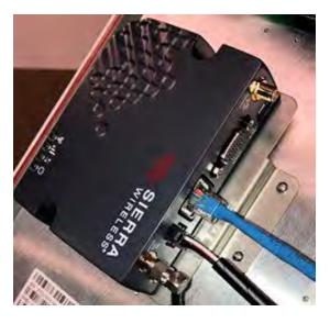
Figure 117 – Reconnect Cables to Sierra Modem
