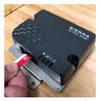
Figure 115 – Insert New SIM Card
