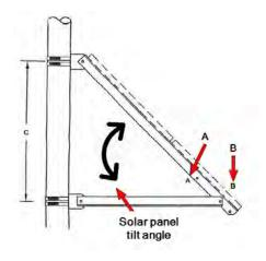
Figure 39 – Solar Panel Tilt Angle
