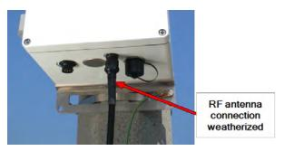
Figure 65 – Weatherized RF Port
