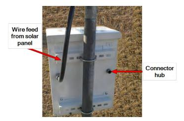
Figure 42 – Back of Battery Box
