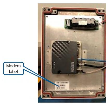
Figure 122 - Check Gateway Door Gasket
