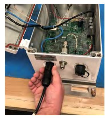
Figure 111 – Disconnect Power to Collector
