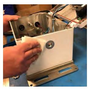
Figure 119 – Clean Antenna Mounting Area
