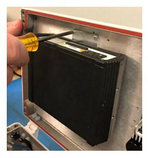
Figure 113 – Removing the Modem
