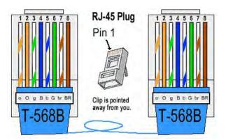
Figure 107 – Straight-Through Ethernet Cable
