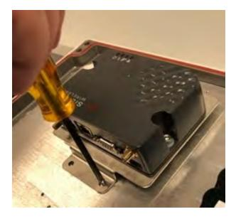
Figure 116 – Mount Sierra Modem on Gateway Door Panel
