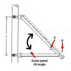
Figure 62 – Adjust Tilt Angle
