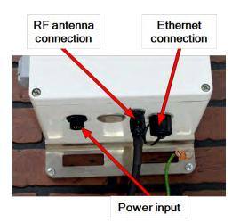
Figure 75 – Adding Gateway Cables
