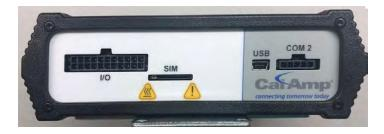
Figure 95 – Modem Back View
