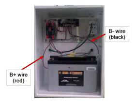
Figure 36 – Battery and Wiring
