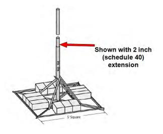
Figure 49 – Concrete Block Ballast
