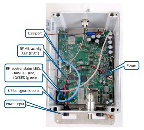
Figure 93 – System LEDs
