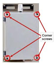
Figure 51 – Gateway Cover Screws
