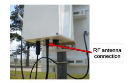
Figure 64 – RF Antenna Cable
