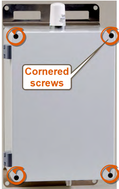
Figure 51 – Gateway Cover Screws
