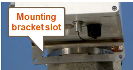
Figure 57 – Slot on Mounting Bracket
