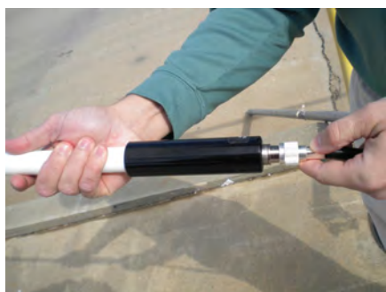
Figure 31 – Attaching Coax Cable
