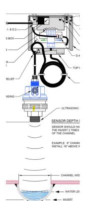
When a Subsonic sensor is used with a SmartCover system, you don't have to worry about losing the signal during a rain event or a surcharge.
